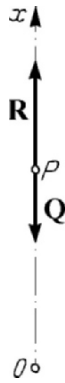
Figure 10.22. Rectilinear motion of a particle of variable mass in a resistent medium.
